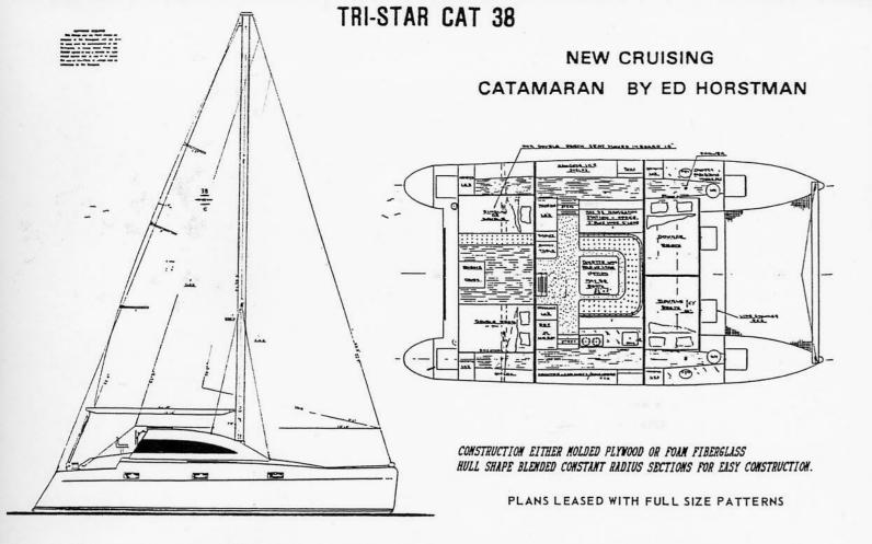
LOA 38'7". LWL 37'7". BEAM 20'6". DRAFT MAIN HULL 28". DRAFT DAGGER BOARD DOWN 5'6". DRAFT RUDDER 36". SAIL AREA 837 FT.SQ. DISPLACEMENT 8800 LB. USEFUL LOAD 4100#. MAIN HULL WIDTH 60".
